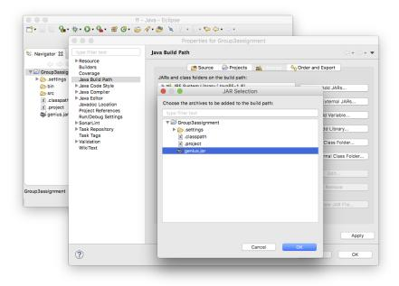
Figure 23: Attach the GENIUS jar to the project.
